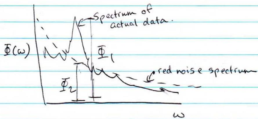
The significance of the ratio  $\Phi_1 / \Phi_2$  can be assessed using the Chi-squared distribution.  $\rightarrow$  test  $\Phi_1$  against theoretical red noise spectrum.
