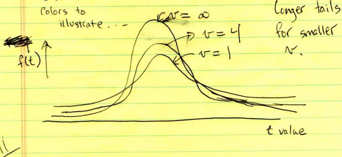
As  $v$  decreases, the distribution gets broader, reflecting the fact it is harder to get a  $t$  value near the tail of the distribution for a small sample size. Approach normal distribution for  $N \sim 30$ , or greater.
