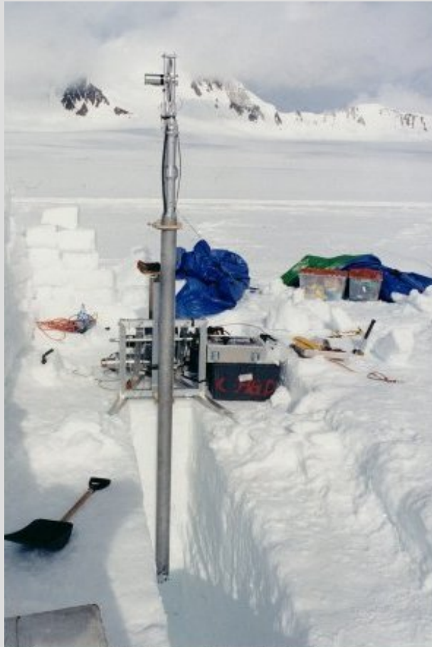
An ice core drill plumbs the depths of a glacier in the St. Elias Mountains, Yukon (photo: Erik Blake)
