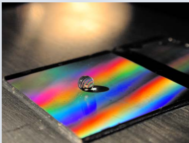
Figure 4. A millimeter-sized water drop at the surface of a textured substrate. The substrate is practically dry even though it supports the drop weight. The regularity of the substrate grooves is evident from its ability to diffract white light. (Courtesy of M. Callies and D. Quéré.)
