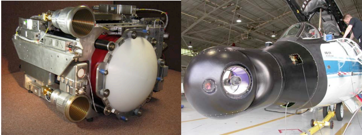
Figure 10: Left: One of the two airborne ATOMMS (Active Temperature, Ozone and Moisture Microwave Spectrometer) transmit and receive modules used as a microwave and Terahertz limb sounder. Right: WB-57F aircraft photograph shows the gymballed nose and in it the present optical imaging instrument that will be replaced by our ATOMMS instrument.
