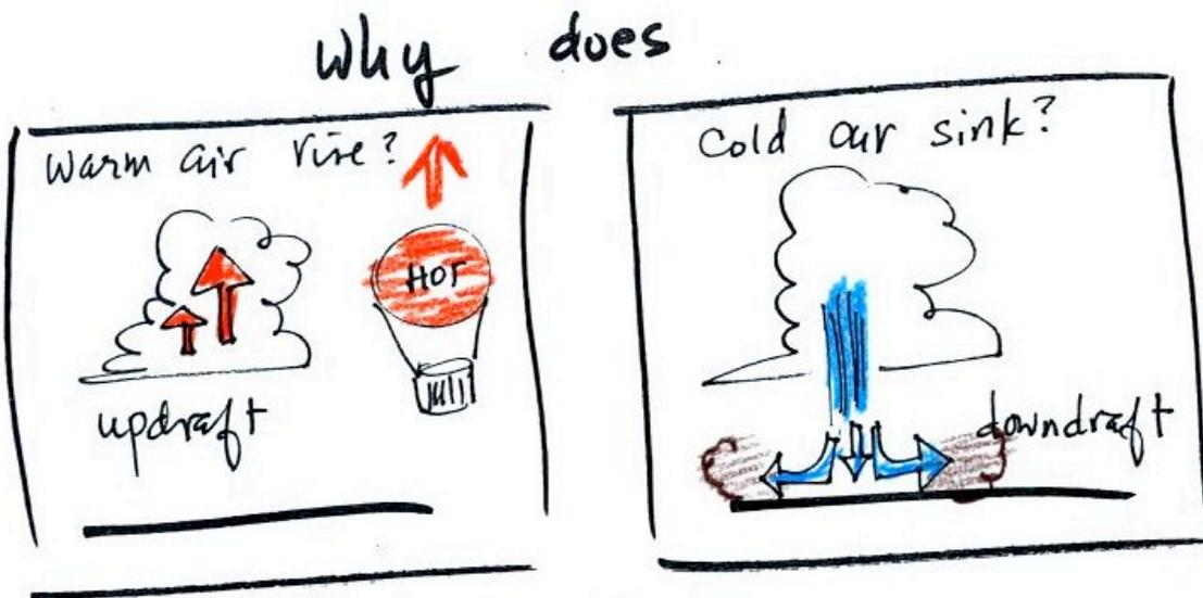
Understanding the ideal gas law is the first step in explaining what actually causes air to rise or sink. The ideal gas law equation is another way of thinking about air pressure on a microscopic scale view. We ignore the atmosphere and instead concentrate on just the air inside a small volume or balloon or parcel of air. We are going to "derive" an equation that shows how pressure (P) depends on certain properties of the air inside the balloon. The word "parcel" means a small volume of air.
