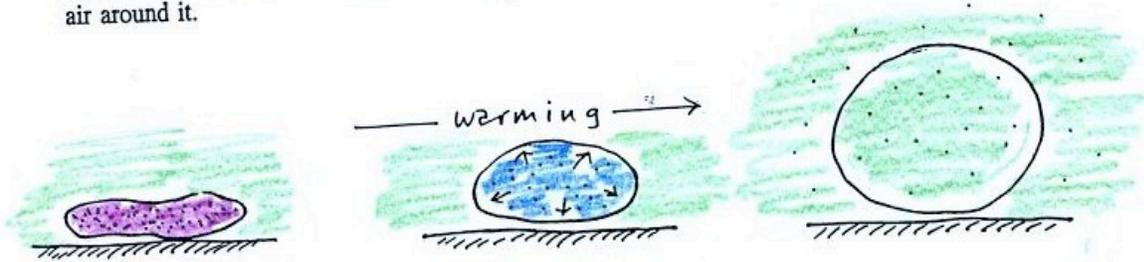
Once we remove the balloon from the liquid nitrogen it will begin to warm and we will be able to see the process in reverse. The air warms, its density decreases, but the air pressure remains constant.
