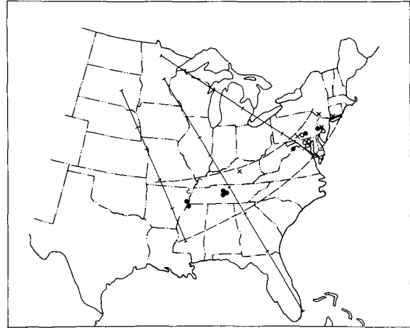
Fig. 13. Zone of small Richardson number diagnosed from isentropic cross sections. Data are from 6 February 1975, 1200 GMT. Turbulence reports are indicated as follows: moderate to severe or severe turbulence (crosses); moderate turbulence (solid circles); and light or light to moderate turbulence (open circles).
